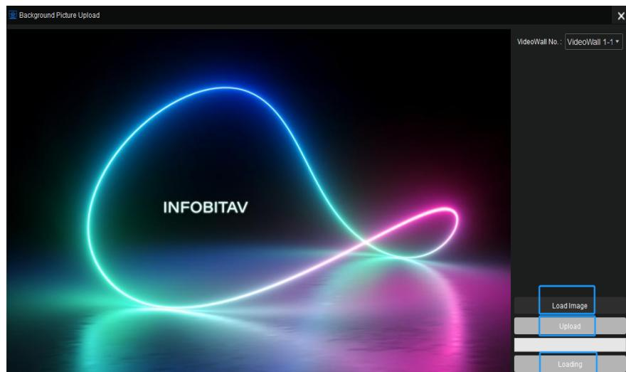
Select the videowall group number. Then load the HD image and click '**Upload**'. When the upload is finished, click '**Loading**' and finally reboot the device.
